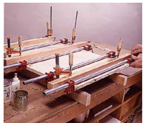
3--Glue and clamp the top using cauls above and below. Wax the cauls to prevent glue from sticking to them.
