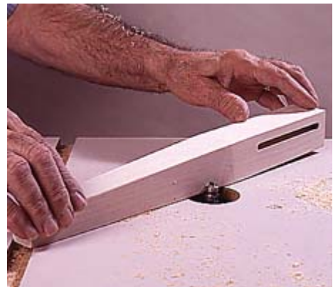
6--Round the bottom of the leg corners on the router table. Don't round the top of the leg where it abuts the apron.
