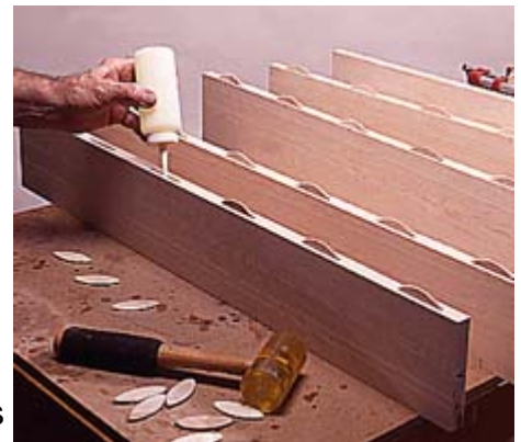
2--Save glue application time by pregluing the joining plates in their slots. A small-nozzle bottle is handy here.
