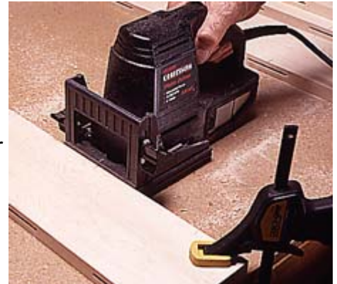
1--Joint the edges of the boards for the tabletop and cut the slots in them to receive the joining plates.
